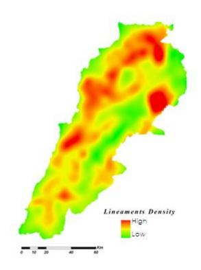
Figure 3-4 Fault - Lineament Density Map
